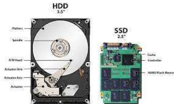
Fig 2: Flash memory and Magnetic Disk
